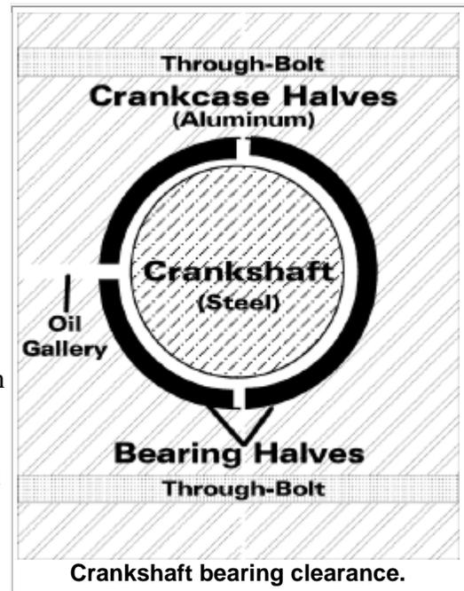
How significant is this problem. Well, engines used in many Cessna singles, the overhaul manual lists the minimum crankshaft bearing clearance as 0.0018 inch (that's 1.8 thousandths) at normal room temperature.
