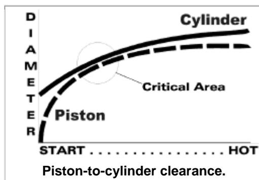
This problem is made worse by the fact that most cylinder barrels are designed with a taper or "choke" in the top one-third of piston travel. This is done to pre-compensate the barrel for the fact that, as the engine comes up to operating temperature, the top of the cylinder (where the combustion process takes place) is a lot hotter than the bottom of the cylinder, and therefore expands considerably more. If cylinders were perfectly cylindrical at room temperature, then
