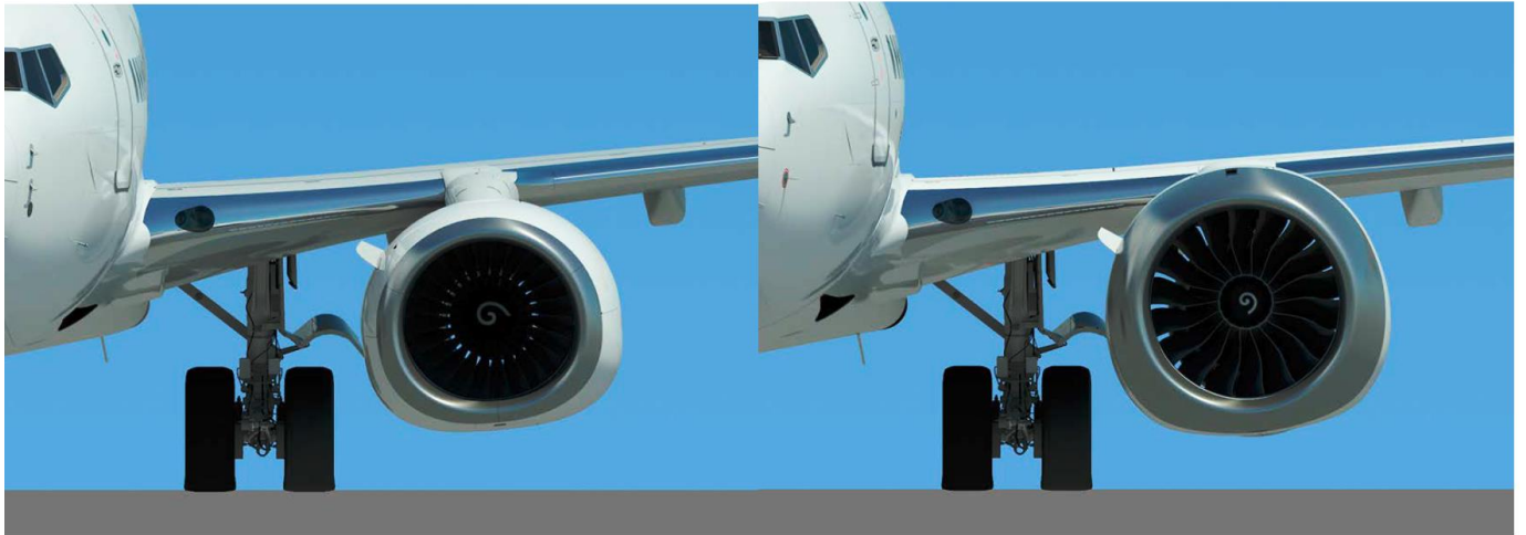
Boeing 737NG (left) and MAX (right) nacelles compared. Source: Boeing 737 MAX brochure.
